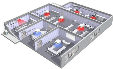
In the Science & Technology Building, we funded the replacement of obsolete digital controls with new, upgraded building automation system (BAS). This will allow improved monitoring and scheduling of the HVAC system and we will be able to schedule the buildings based on occupancy levels.
