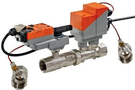
ECU purchased and installed energy valves on all major air handling units served by Central Chiller Plant #1. The energy valves ensure that we optimize the chilled water flow through the coil; thereby ensuring maximum efficiency and savings on electricity for pumping.
