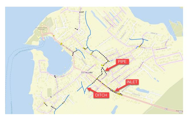
Figure 20: Approximate Drainage Mapping Completed During RCCP
